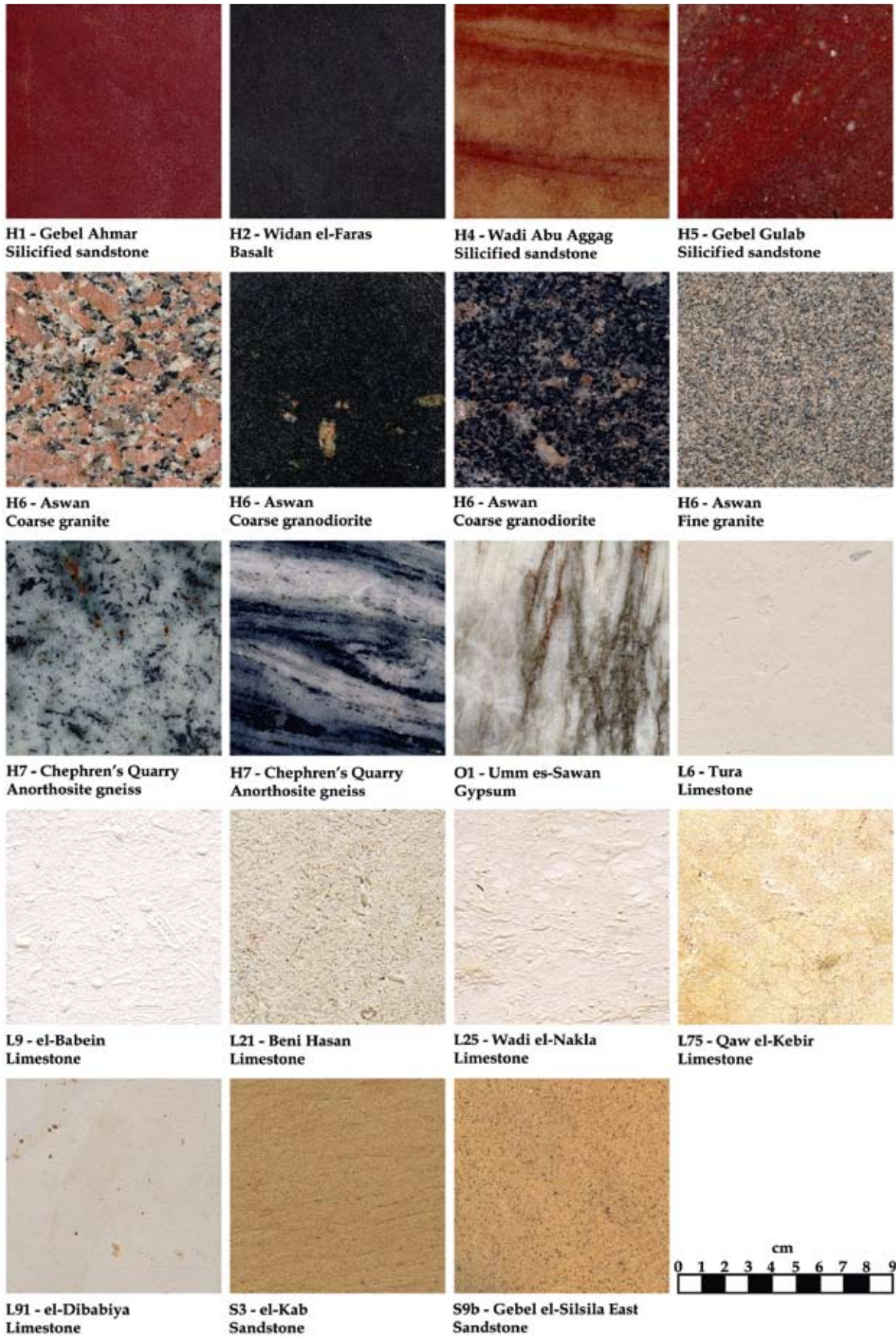
Figure 10. Selected stones from ancient quarries in the Nile Valley and Western Desert. The numbering and sequence of the images follow the list of quarries on the reverse side of the attached, fold-out map. Not all quarries and rock varieties are represented. Photos by James Harrell.
