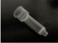
Empty spin columns are convenient for cleaning DNA with PVPP or any customized matrix.
