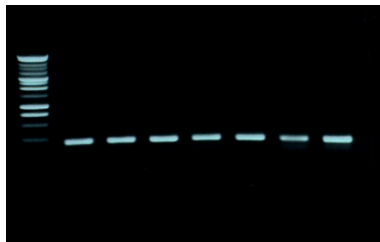
PCR products (180 bp) on an agarose gel. A DNA ladder is shown in the first lane
