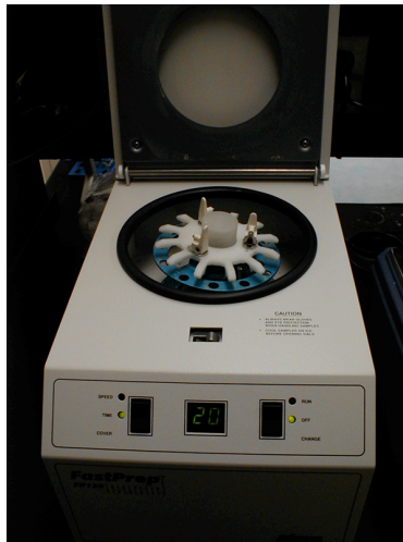
A bead-beater rapidly shakes microcentrifuge tubes that contain sample and glass beads to lyse cells and release DNA.
