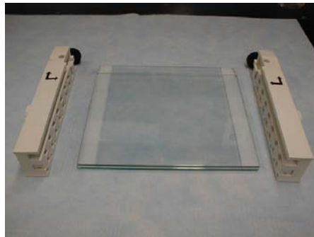
Components of the gel sandwich; gel clamps and spacers between two glass plates.
