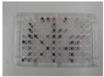
Example of a BIOLOG plate inoculated with a dilution of soil and incubated for 48 hours. The purple wells contain carbon sources that were used by the microbial community. The intensity of the purple coloration indicates the degree of carbon source usage by the community.
