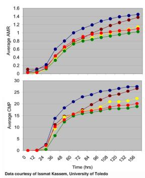
CLPP profiles comparing the AMR and CMD of five classes of lake bottom sediments. Sediment classes: freshly dredged (red line), sampled from open lake-disposal site (green line), surface stored for 20 years (blue line), 5 years (brown line) and less than one year (yellow line).
