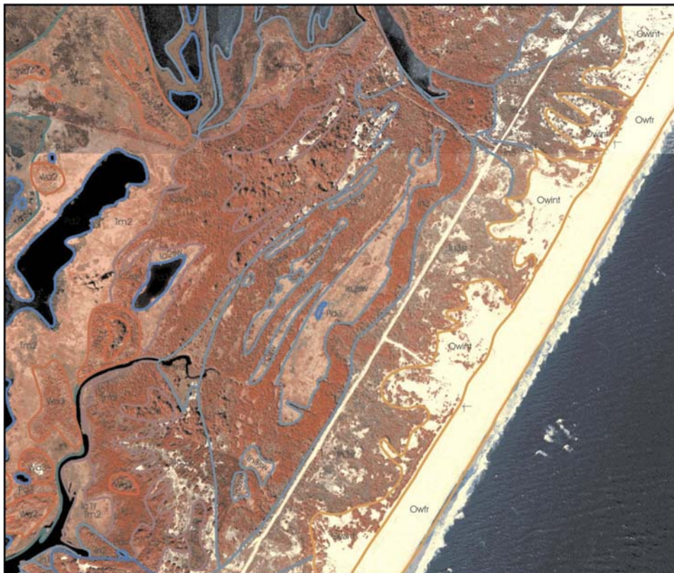
Figure 15. Inlet-closure ridges and intervening swales at the former Green Run Inlet. Near kilometer 33.
