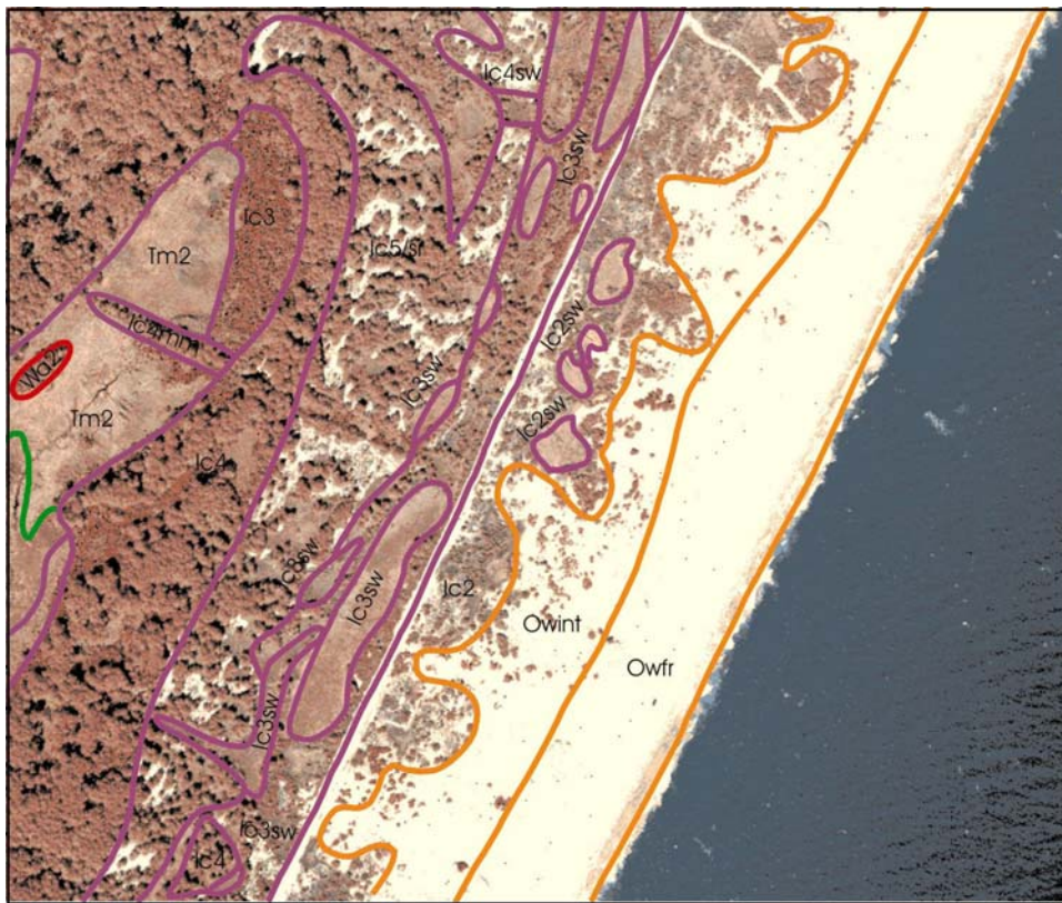
Figure 14. Ocean-side swales that receive seawater overwash intermittently. Classified as IC3sw or IC2sw depending upon the relative frequency of inundation by seawater. These swales have a unique salt-tolerant grass community dominated by Spartina patens , Distichlis , and Juncus . Near kilometer 29.
