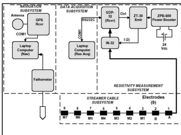
Figure 2. Schematic diagram for streamer resistivity configuration (adapted from Snyder and Wightman 2002).
