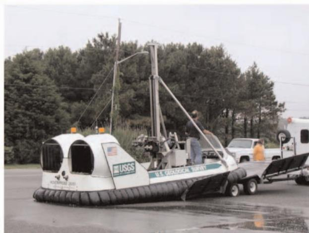
**Figure 4.** Hoverprobe deployment at Public Landing (Chincoteague Bay), Maryland. Hoverprobe is self-launching into boat ramps.
