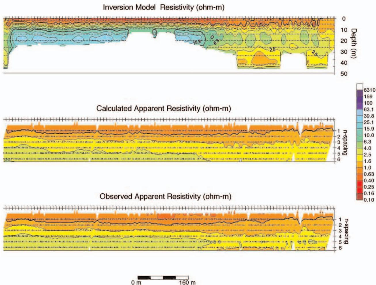
**Figure 3.** Triad of resistivity profiles for Delaware Line 3, produced by Zonge Co. using TS2DIP and Surfer software. The lower two pseudosections (dipole/resistivity plots) represent observed resistivity (bottom) and calculated observed resistivity (middle). The top section depicts the interpreted resistivity contours plotted against depth (inversion model).
