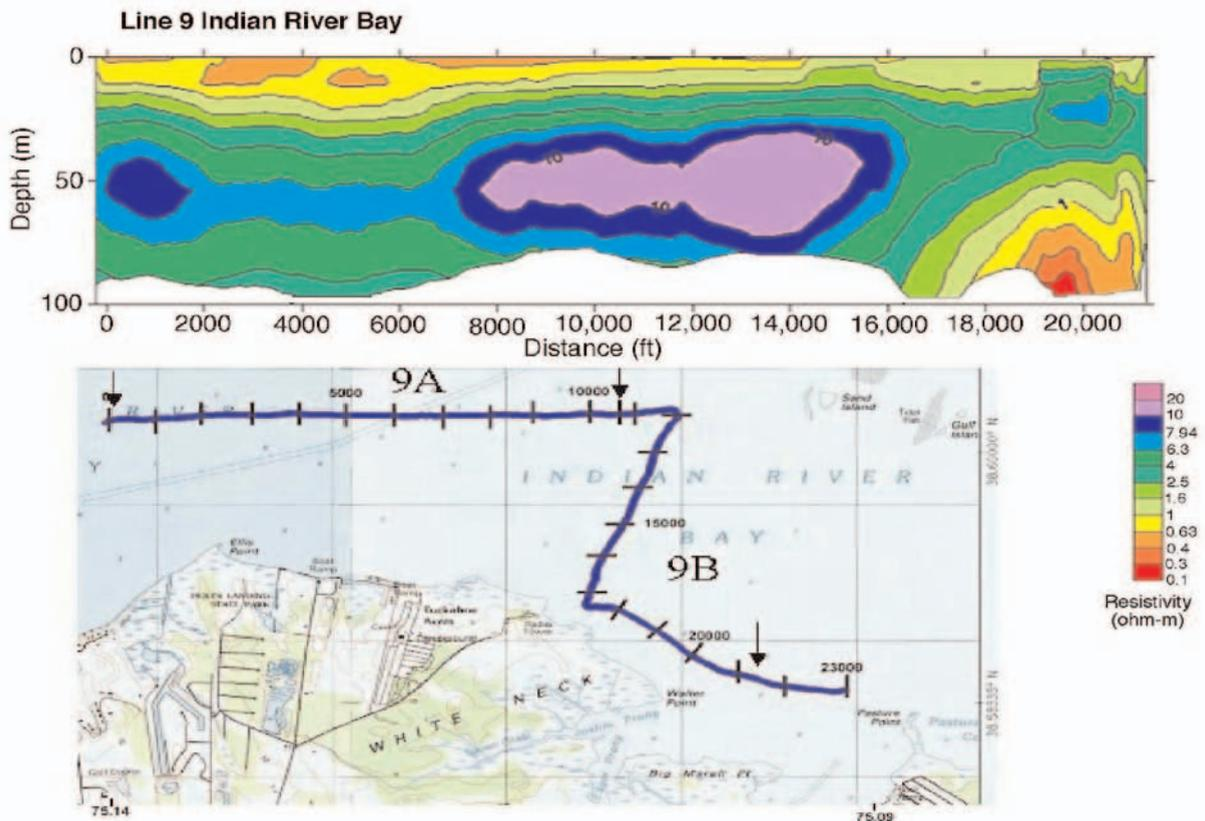
Figure 8. Resistivity Line 9 from Indian River Bay. Note that the line takes a right angle turn at ~10,800 ft from origin.
