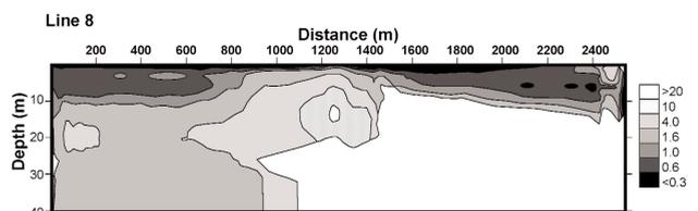
Figure 12. Resistivity Line 8 from Chincoteague Bay transverse to Line 1. The interpreted profile is corrected for water-column effect (see Figure 6 caption).
