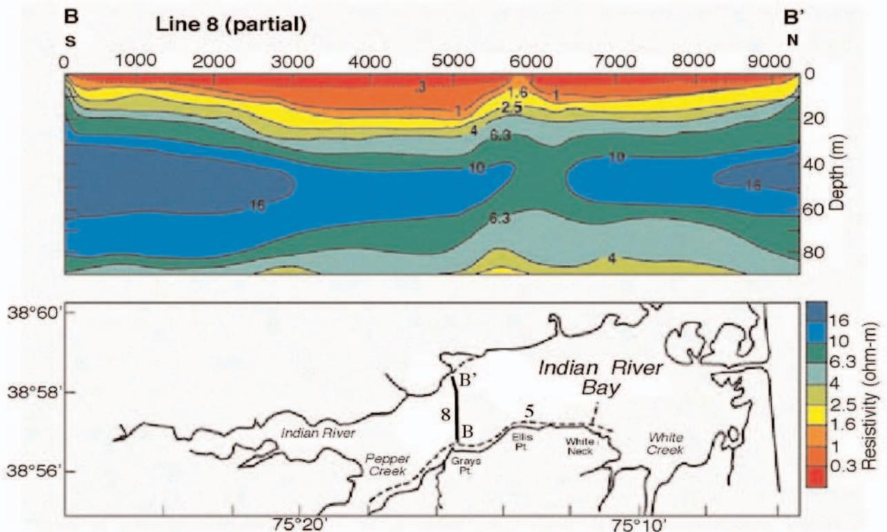
Figure 7. Resistivity Line 8 from Indian River Bay. Locations are shown in a plot beneath the profile. The profile was redrawn manually from initial high-resolution Surfer output.
